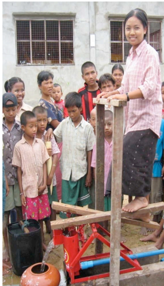
A simple treadle pump brings water to the surface at a school in Southern Asia.
